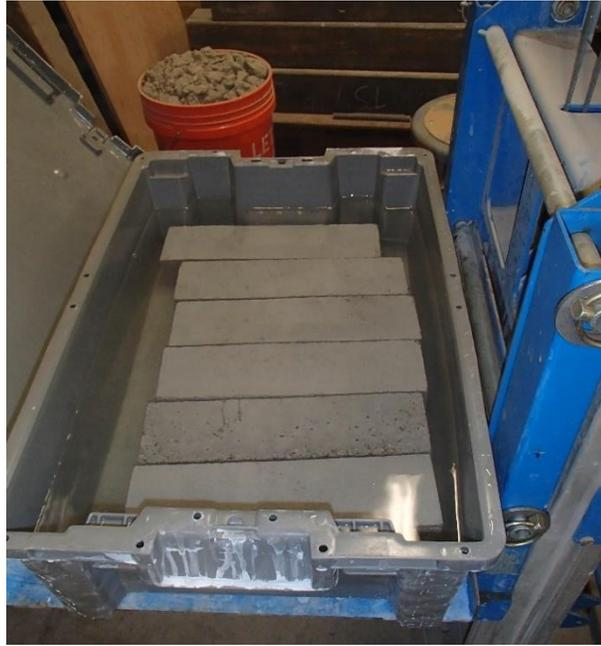
Figure 4-22: ASR Specimens Submerged in Sodium Hydroxide Solution
