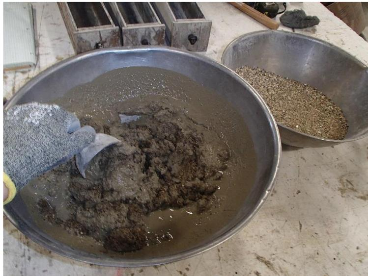
Figure 4-20: Hand Mixing the Mortar for ASR Testing
