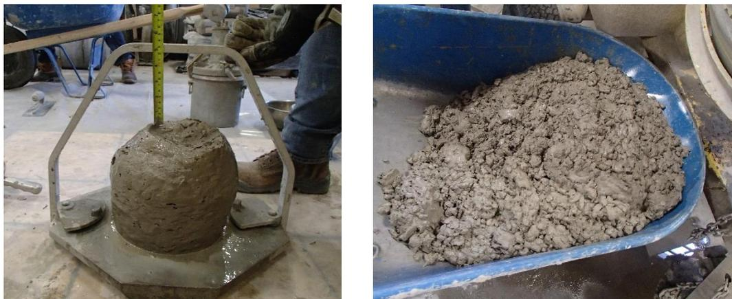
Figure 5-4: Example of MIX 6-HD with Stiff Consistency
