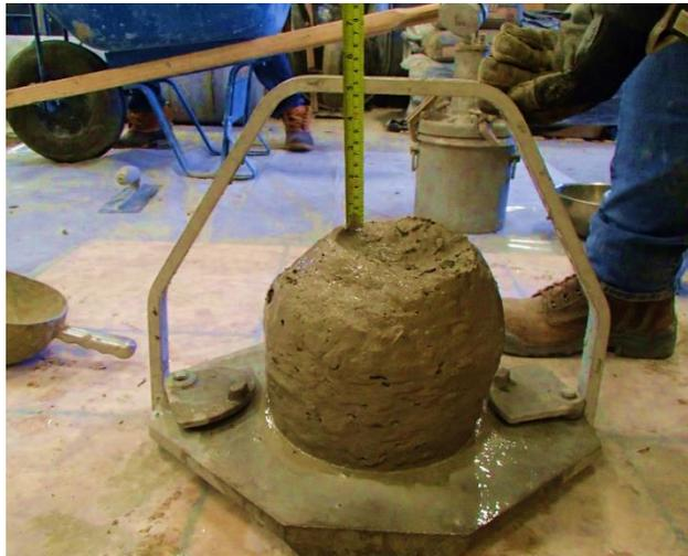
Figure 4-8: Measuring the Slump of a Concrete Mixture
