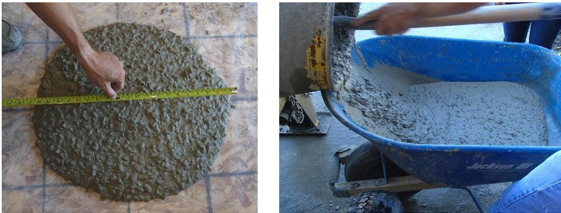
Figure 5-3: Example of MIX 6-HD with Flowable Consistency
