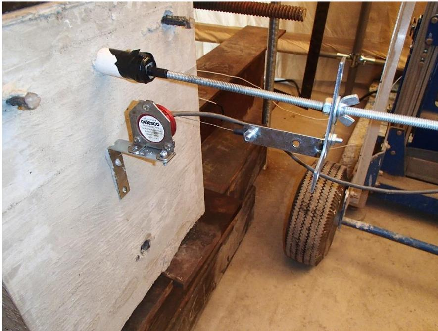
Figure 4-28: Apparatus Used for Measuring Slip During Bar Pullout Test
