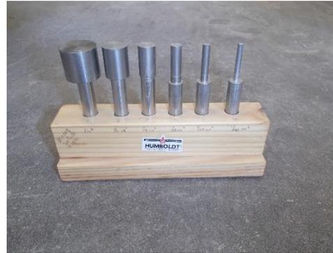
Figure 4-12: Acme Penetrometer Used to Measure Initial and Final Set Time of Concrete Mixtures & Various Penetrometer Needle Sizes
