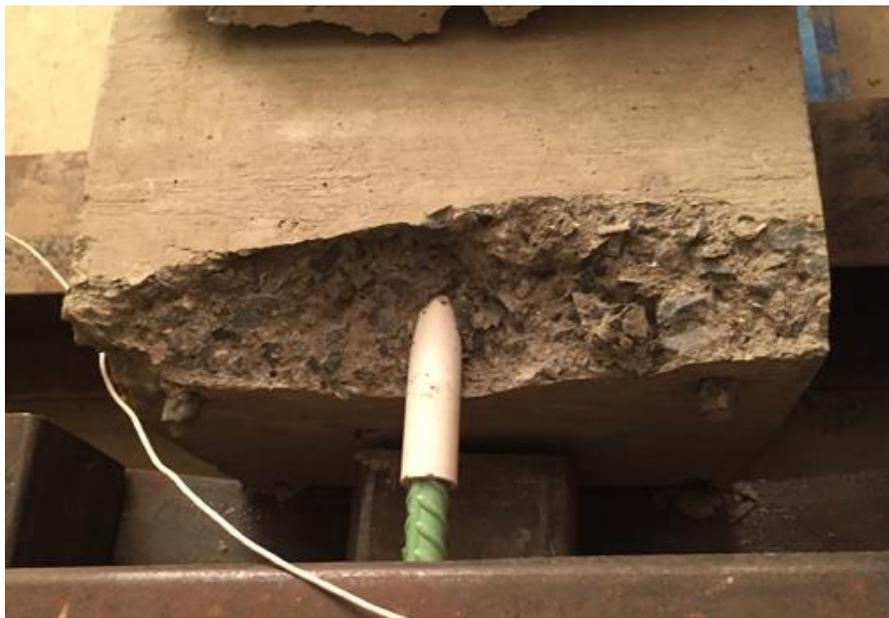
Figure 5-15: Concrete Cracking of Test Specimen 15-HD-6
