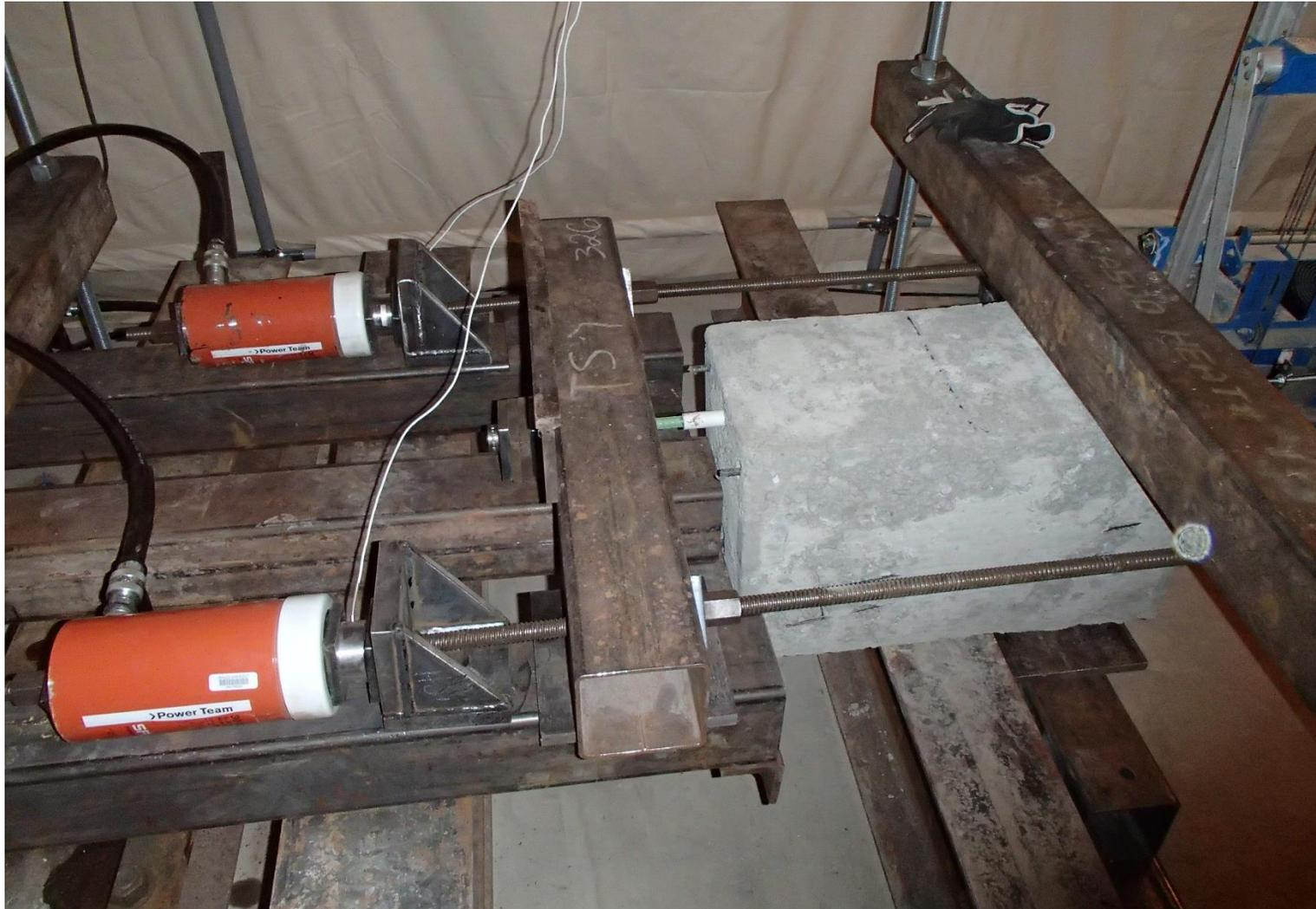
Figure 4-31: Bar Pullout Test Apparatus
