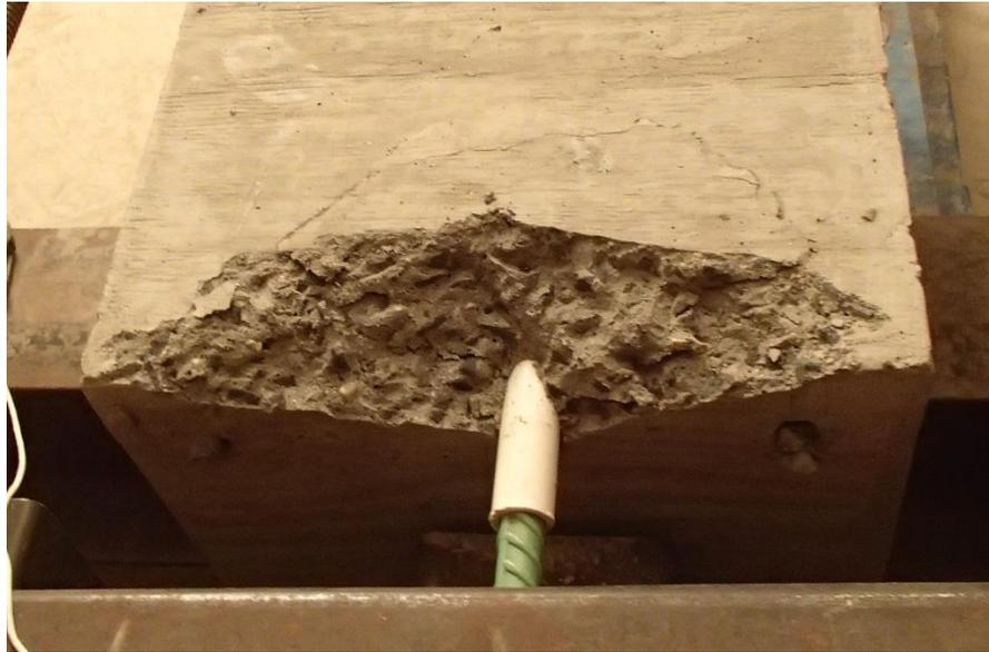
Figure 5-14: Concrete Cracking of Test Specimen 6-HD-6
