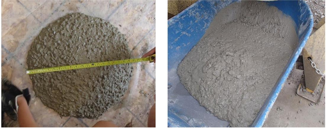
Figure 5-5: Example of MIX 15-HD with Flowable Consistency
