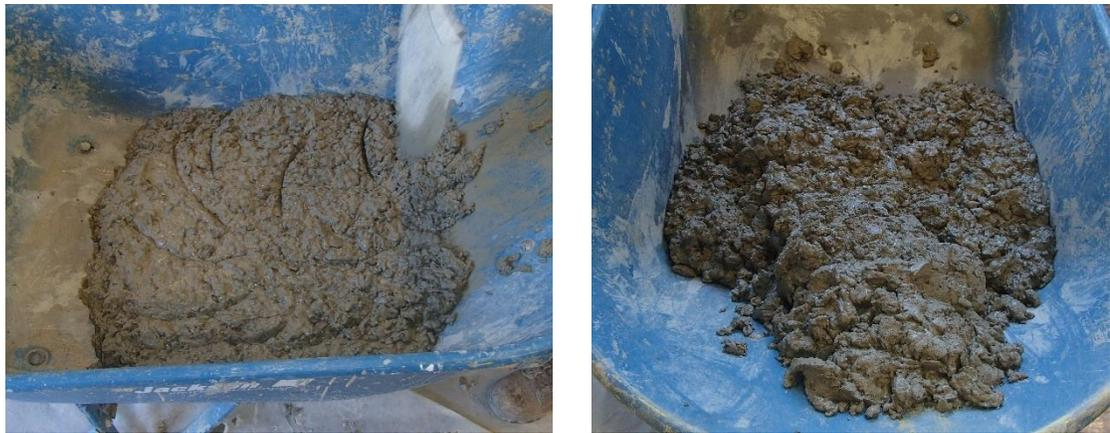
Figure 5-6: Example of MIX 15-HD with Stiff Consistency
