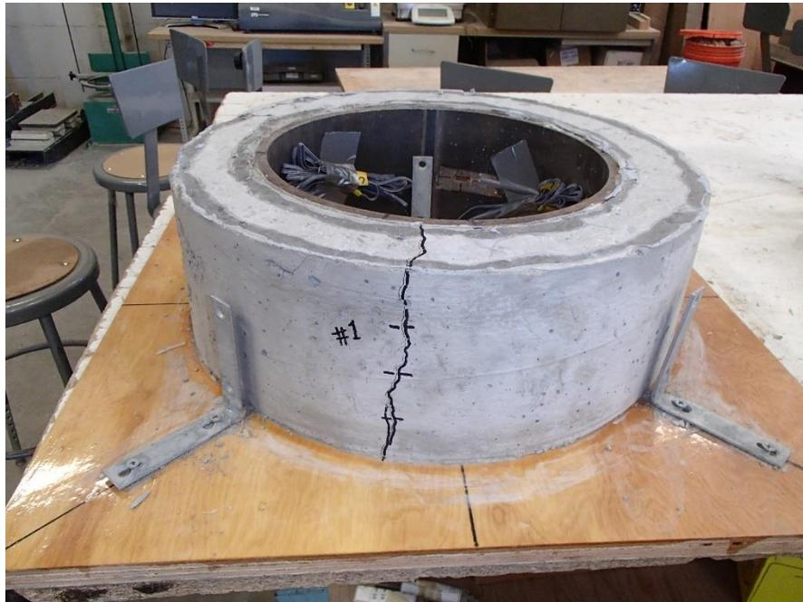
Figure 5-18: Typical Crack Formation in a Confined Shrinkage Ring
